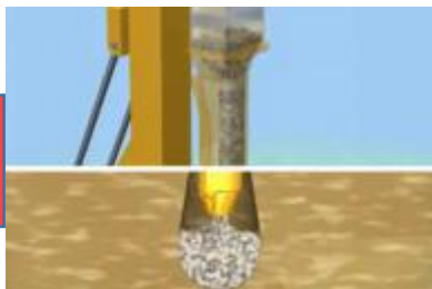
Stone go into soil from pipe
